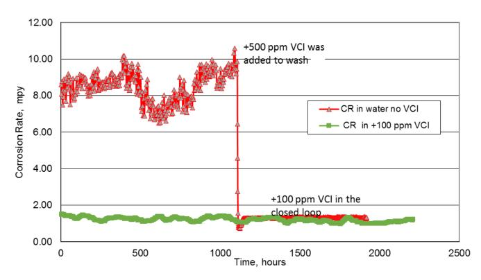
Figure 4: Comparison of corrosion rate measurements of the inhibitor treated loop and control test after 2,200 hours corrosion test in hot steam/water closed loop.
