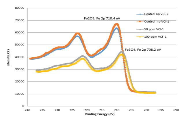
Figure 7: High Resolution XPS analysis on the inner pipe surface after corrosion test in the hot steam loop. Primary oxide seen on ID surface of non-treated pipes (control) is hematite, while magnetite is predominant oxide on ID surface of VCI treated pipes.
