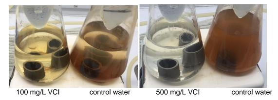
Figure 2: Corrosion behavior of the steel pipe samples in boiling water. Corrosion rate decreased to 1.36 mpy with 100 and 500 mg/L VCI addition, (700 hours).
