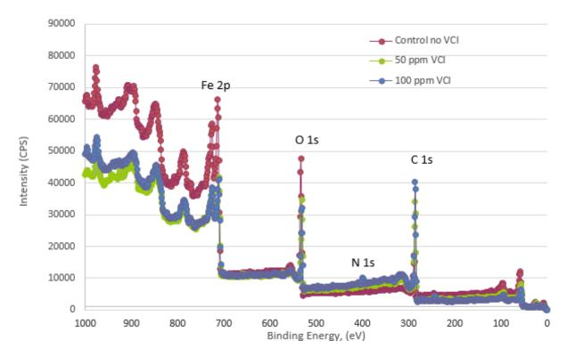
Figure 6: XPS analysis on the inner pipe surfaces after corrosion test in the hot steam loop shows more corrosion product on the control test.
