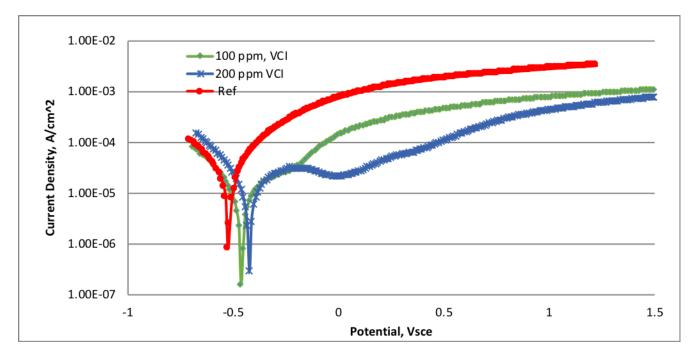
Figure 1: Comparison of cyclic polarization behavior of steel pipe in hot water solution in 100°C when exposed to control solution, 100 and 200 mg/L VCI.
